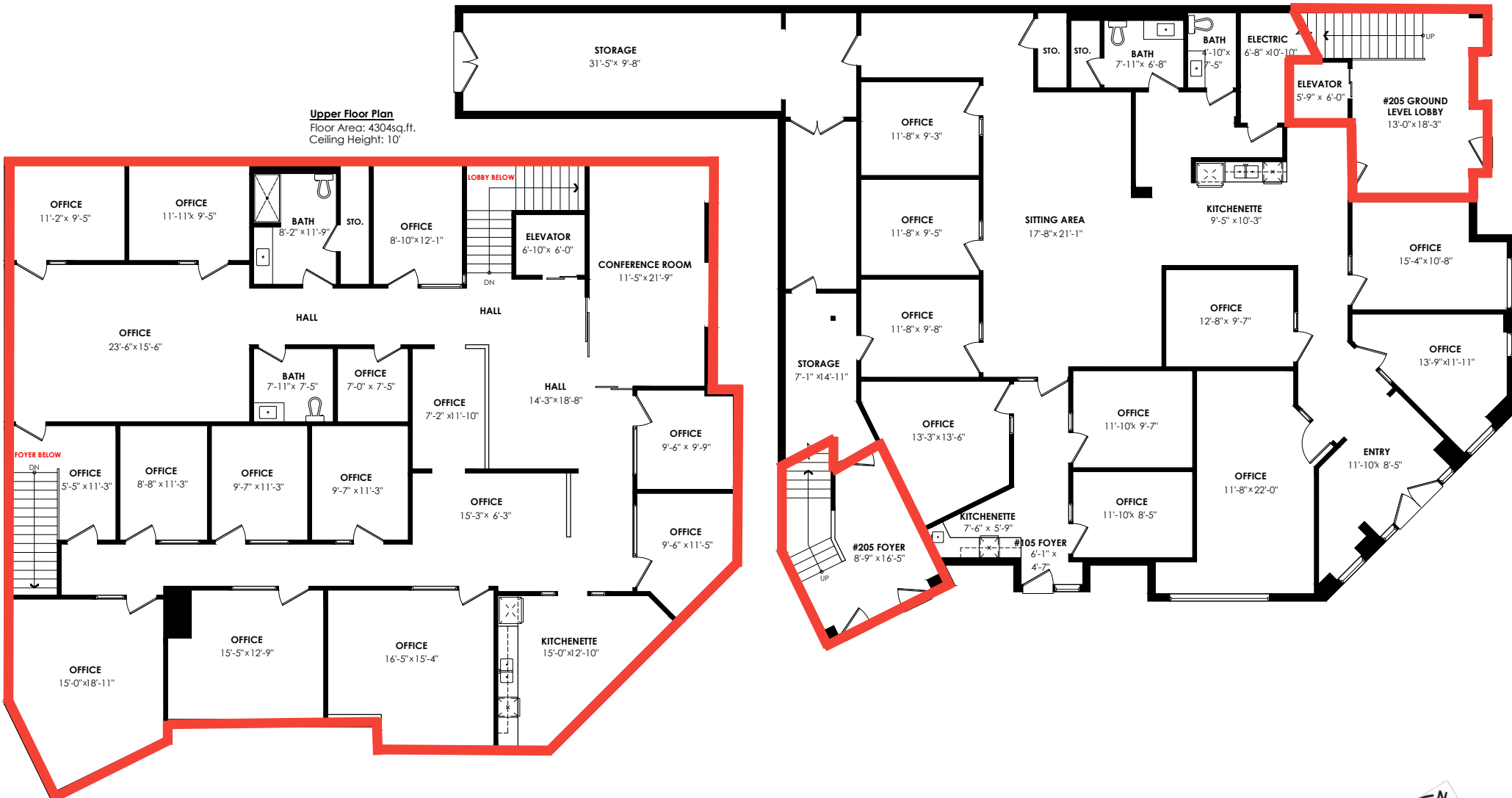
Main Floor Plan Floor Area: 3671 sq. ft. Ceiling Height: 11'
