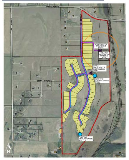
Concept services provided by a communal potable water and & wastewater treatment plant in accordance with the Municipal Development Plan which includes:
