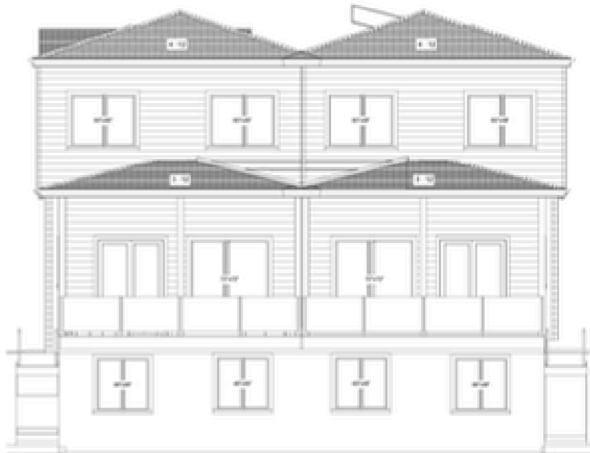
Exterior Elevation Back
